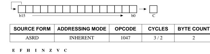
This instruction shifts the contents of Accumulator D to the right by one bit. Bit 0 is shifted into the Carry flag of the Condition Codes register. The value of bit 15 is not changed.
