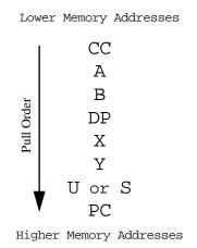
For each 8-bit register specified, a byte is read from the memory location pointed to by the stack pointer and then the stack pointer is incremented by one. For each 16-bit register specified, the register's high-order byte is read from the address pointed to by the stack pointer and then the stack pointer is incremented by one. Next, the register's loworder byte is read and the stack pointer is again incremented by one.
