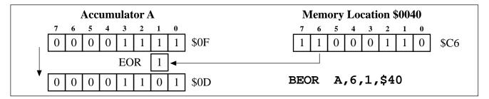
The figure above shows an example of the BEOR instruction where bit 1 of Accumulator A is Exclusively ORed with bit 6 of the byte in memory at address 0040 (DP = 0).
