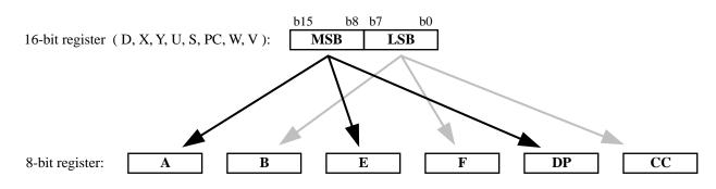
The TFR instruction requires a postbyte in which the source and destination registers are encoded into the upper and lower nibbles respectively.
