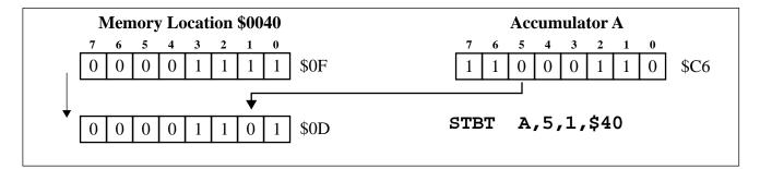
The figure above shows an example of the STBT instruction where bit 5 from Accumulator A is stored into bit 1 of memory location 0040 (DP = 0).
