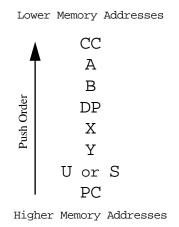
For each 8-bit register specified, the stack pointer is decremented by one and the register's value is stored in the memory location pointed to by the stack pointer. For each 16-bit register specified, the stack pointer is decremented by one, the register's low-order byte is stored, the stack pointer is again decremented by one and the register's high-order byte is then stored.
