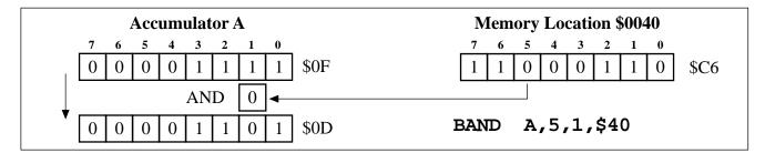
The figure above shows an example of the BAND instruction where bit 1 of Accumulator A is ANDed with bit 5 of the byte in memory at address 0040 (DP = 0).
