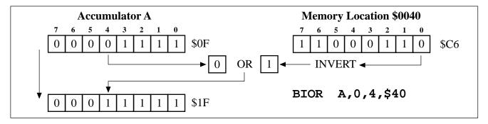
The figure above shows an example of the BIOR instruction where bit 4 of Accumulator A is logically ORed with the inverted value of bit 0 from the byte in memory at address 0040 (DP = 0).
